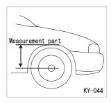
**3.** After installing the tires, measure the distance from the wheel center and the fender edge as shown in the Figure, and confirm that it corresponds to the reference value shown below.
