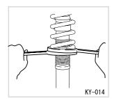
**2.** After adjusting to the appropriate height, use the adjustment wrench included with the Product to lock the lower spring seat.
