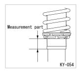
1. After installing the shock absorber on the vehicle, measure the area marked in the Figure, and adjust to match the reference values shown.
