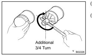
(d) Lightly screw the oil filter into place, and tighten it until the gasket contacts the seat.
