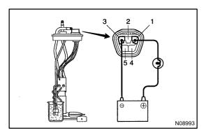
(b) Submerge the switch in fuel, check that the bulb goes out. If operation is not as specified, replace the sender gauge.
