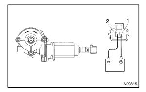
(b) Reverse the polarity, and check that the motor turns clockwise.
