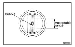
(b) Make sure the gauge bubble is within the acceptable range.
