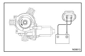
(b) Reverse the polarity, and check that the motor turns counterclockwise.
