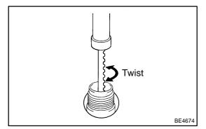
(b) Wind the cable to retract the rod by turning the ignition switch to "LOCK" position.
