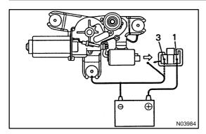
(b) Disconnect the negative (-) lead from terminal 3, check that the motor stops running at the stop position.If operation is not as specified, replace the motor and relay.
