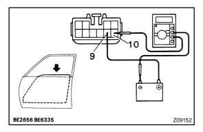
(e) Check that the current increases up to approximately 14.5 A or more when the window stops going down.
