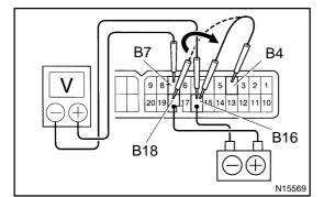
(e) After connecting terminal B4 to terminal B18, connect to terminal it to terminal B16, check the voltage rises from 0 V to battery voltage with in the times, as shown in the table.
