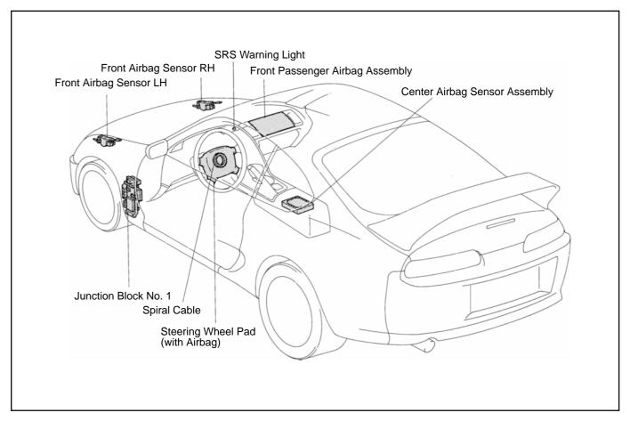
Servicing vehicle with a Supplemental Restraint System (referrerd to as the SRS in the remainder of this manual) installed.
