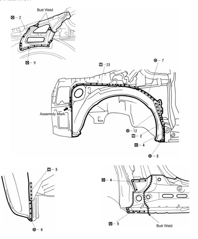
Determine the position of the new parts by the assembly marks of the inner and outer panels.
