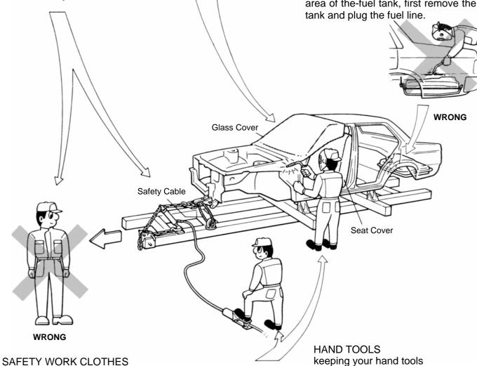
In addition to the usual mechanic's wear, cap and safety shoes, the appropriate gloves, head protector, glasses, ear plugs, face protector, dust-prevention mask, etc. should be worn as the situation demands.
