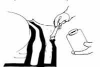
Remove the paint from the portion of the new parts and body to be welded, and apply weld-through primer. HINT: See "ANTI-RUST TREATMENT" on page AR-2.
