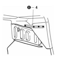
1. Push down on the rear floor pan to quarter panel extension and remove it.
