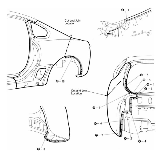
Cut and join the parts at the location shown above.
