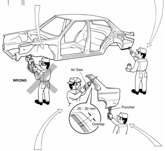
ROUGH CUTTING OF JOINTS For joint areas, rough cut the new parts, leaving 20 - 30 mm (0.79 - 1.18 in.) overlap.
