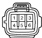
Fig. 2: Front Wiper Motor Terminals (Avalon, Celica, Corolla, RAV4, Supra & T100)
