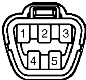
Fig. 8: Fuel Sending Unit Wiring Harness Connector Terminals
